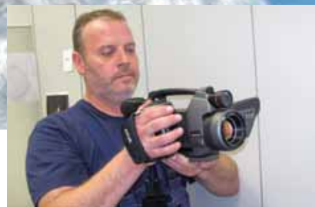
Maintenance engineer Thorsten Krämer uses the FLIR P620 to inspect a fuse cabinet.
