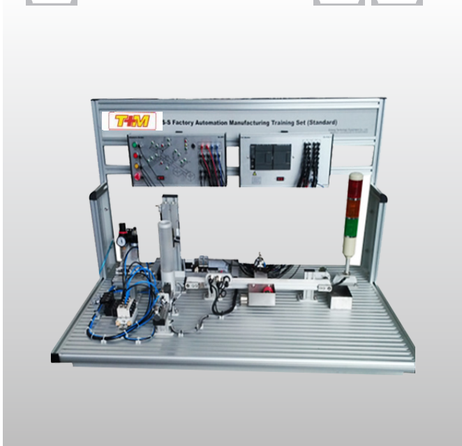
DLFA-MAS-S Factory Automation Manufacturing Automation System
