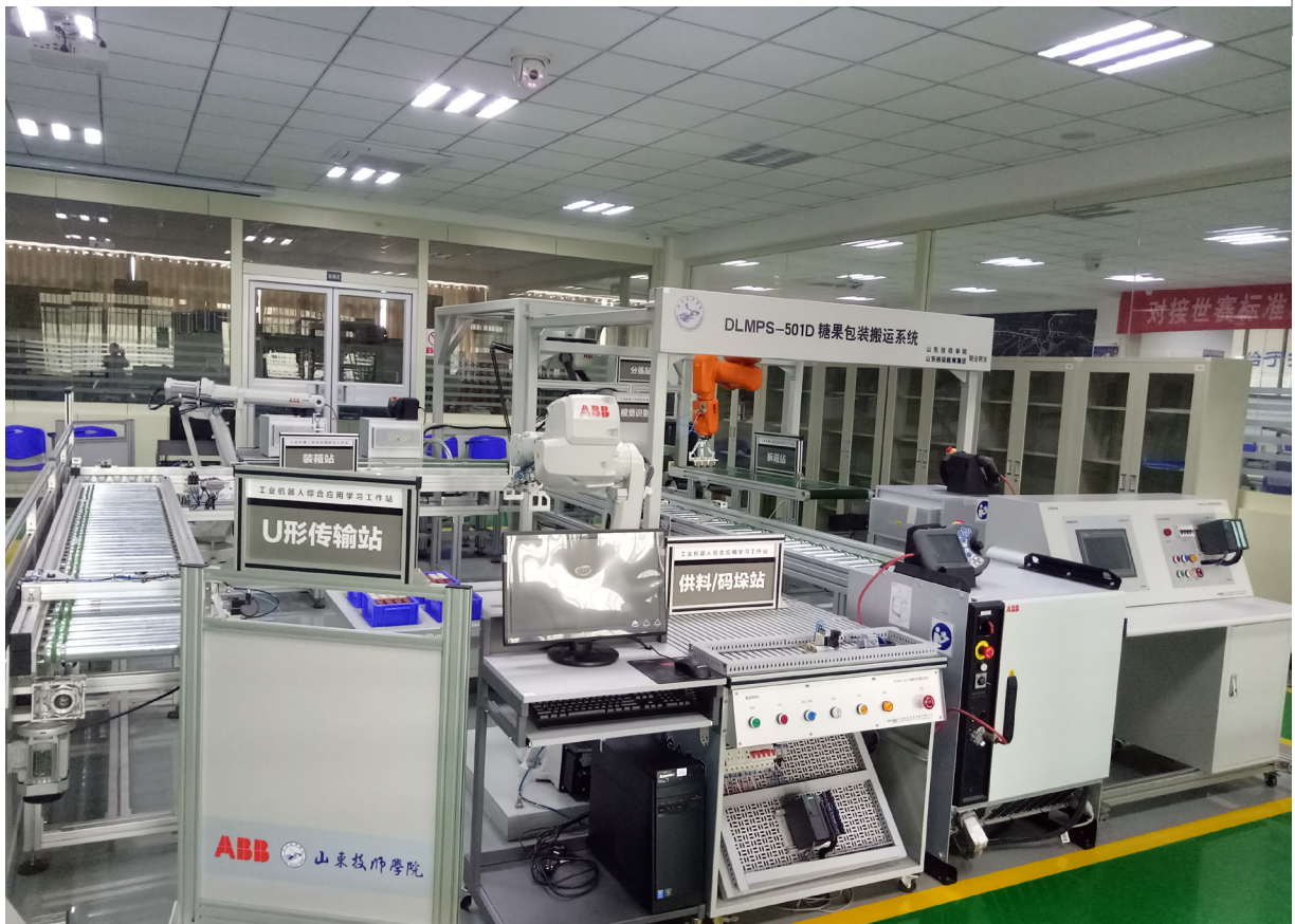
DLMB-501D Industrial robot candy packaging and handling system
