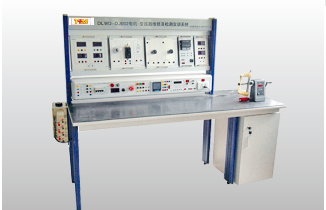
DLWD-DJB02 Motor &amp; Transformer Maintenance &amp; Test Training System
