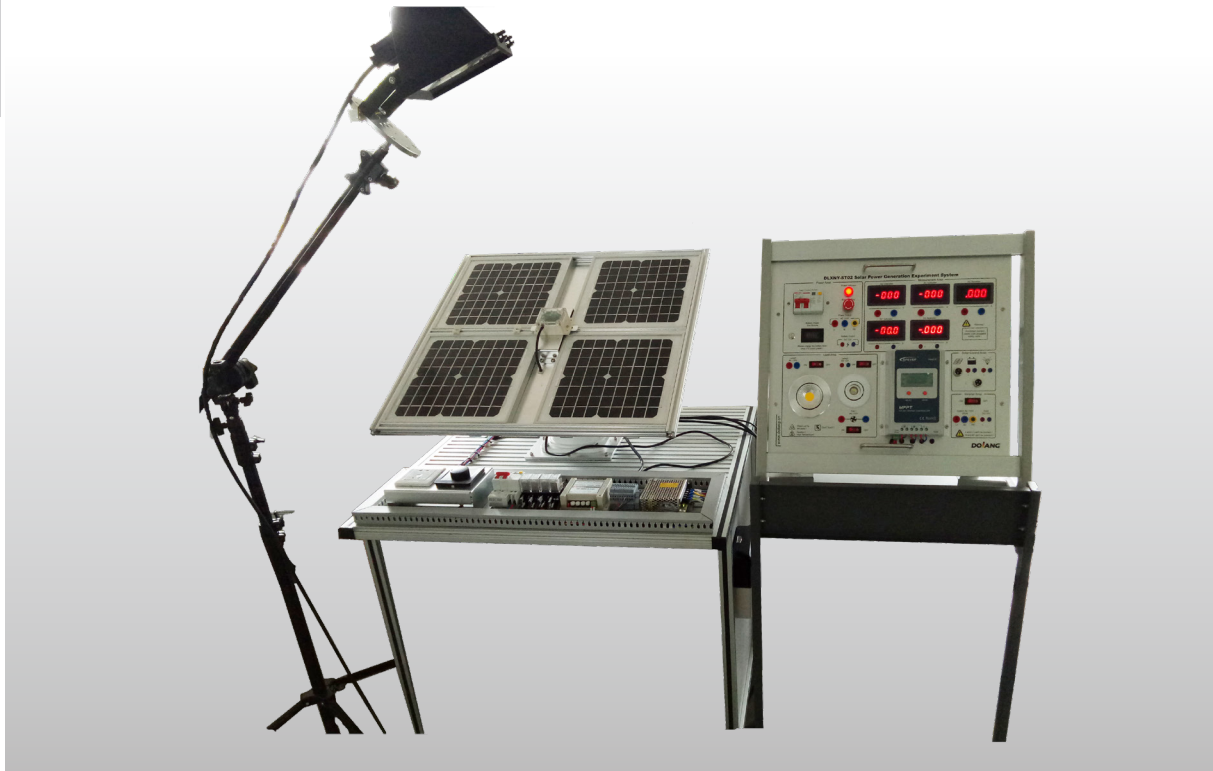
DLXNY-ST02 Solar Power Generation Experiment Platform
